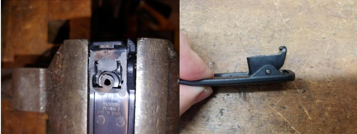
Next, use a 5/16" drill to put roughly 1/16" deep recess in the area where the screw hole is to match the circular portion of the "key notch" on the radio
