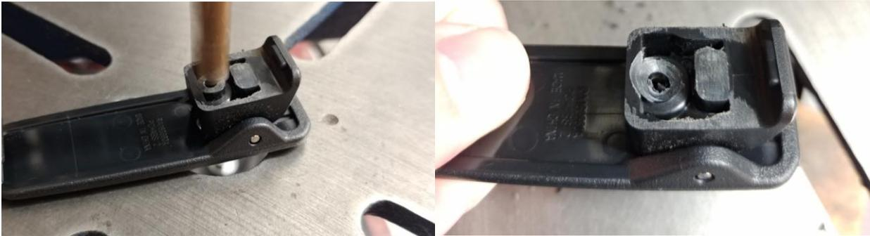
Now, back in a vice I used a small chisel to knock a small notch in the middle of the flat rectangular part to fit the upper portion of the "key notch" in the back of the radio.
