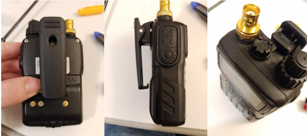
One final note, if you use the drop-in charger it will now be necessary to depress the spring clip before it can insert into the dock.
